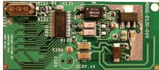
26mm x 59mm CX86500 Modem Reference Design
